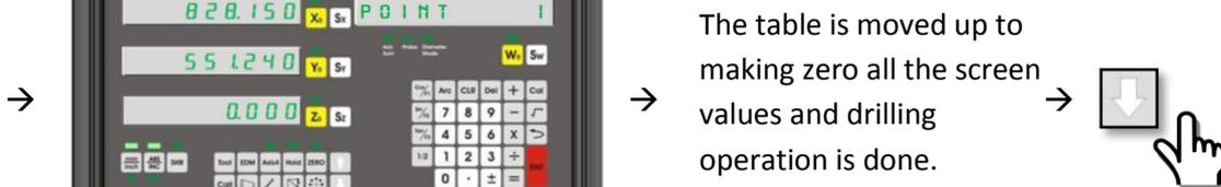
→ Point 2 values are screened. The table moved up to making zero all axis values and drilling operation is done. By ↓ button the following point is passed. For all points the same operations are done.
