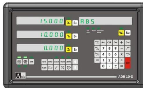
→ When you move up to reset axis value zero you can find the centre of the work piece.
