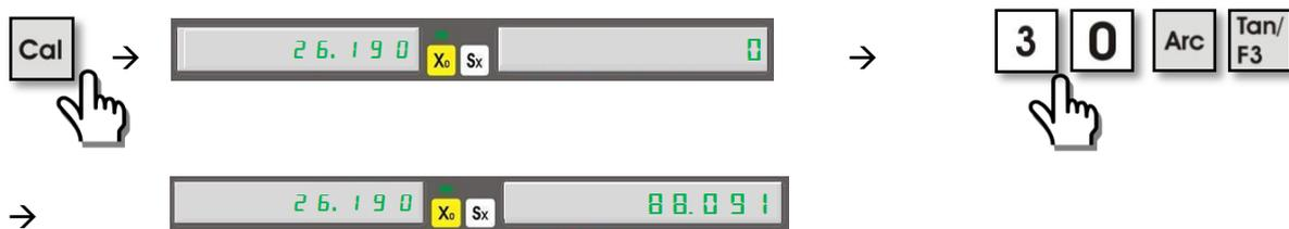
**5.6.1. To Transfer the Calculated Values to the Axes:** The calculated values can be transfer to the axes. After calculation please press
