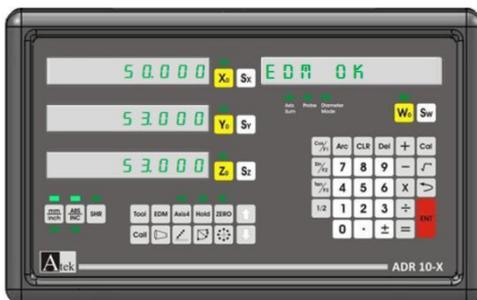
When 50 mm + 3 mm (Offset) depth value is received the relay changes its position and digital readout warns the user both by written and sounds. To exit press EDM button or enter or
