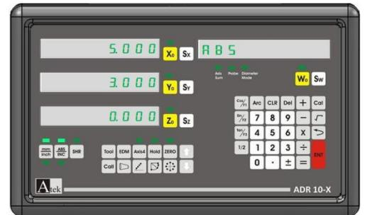
When the work pieces are moved up to make zero all axes you will find the work piece centre.
