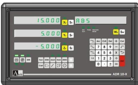
After turning to ABS screen, when you add 5 mm for each axis:
