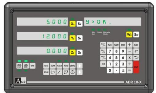
**Tool Memory Setting Second Way (Manuel):** Move Y axis to zero point.
