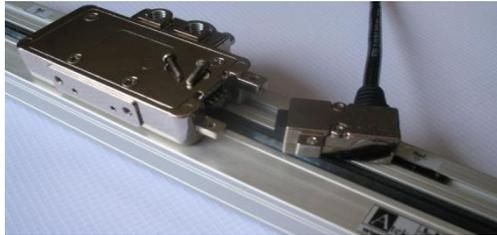
The connector is put on its place. The screws is closed again by Phillips screwdriver. Anymore the cablo is on the other side.
