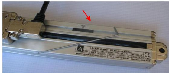
Reference determining's set screw screws are removed to change the reference point with 1,5 mm allen and drifted to the other reference point. Set screw are squeezed again.
